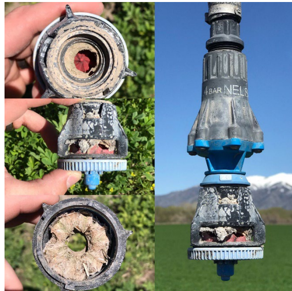
Figure 1. Moss debris clogging pivot sprinkler.
